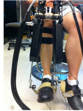
Fig. 1. Experimental setup. Subject wearing Anklebot in a seated posture.
