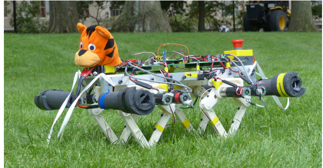
Fig. 1: The Super Mini Cheetah (SMC) quadrupedal robot: a small quadrupedal robot capable of indoor and outdoor behaviors such as walking, hopping, running, turning and stopping. The robot is used in this study to evaluate hopping over hard and soft ground and to measure ground properties in-situ.
