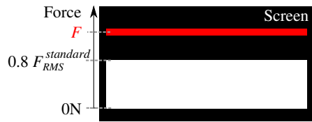
Fig. 3. Online visual feedback of the force applied on the robot provided to participants of Exp.2.B. The red bar moved vertically. F is the current magnitude of the applied force, averaged over 80 ms. F_{RMS}^{standard} is the average RMS force applied by the participant over 10 trials of the standard (biological) condition. The success zone (white rectangle) was smaller than F_{RMS}^{standard} so that participants would not be tempted to plateau when they reached the level of F_{RMS}^{standard} .
